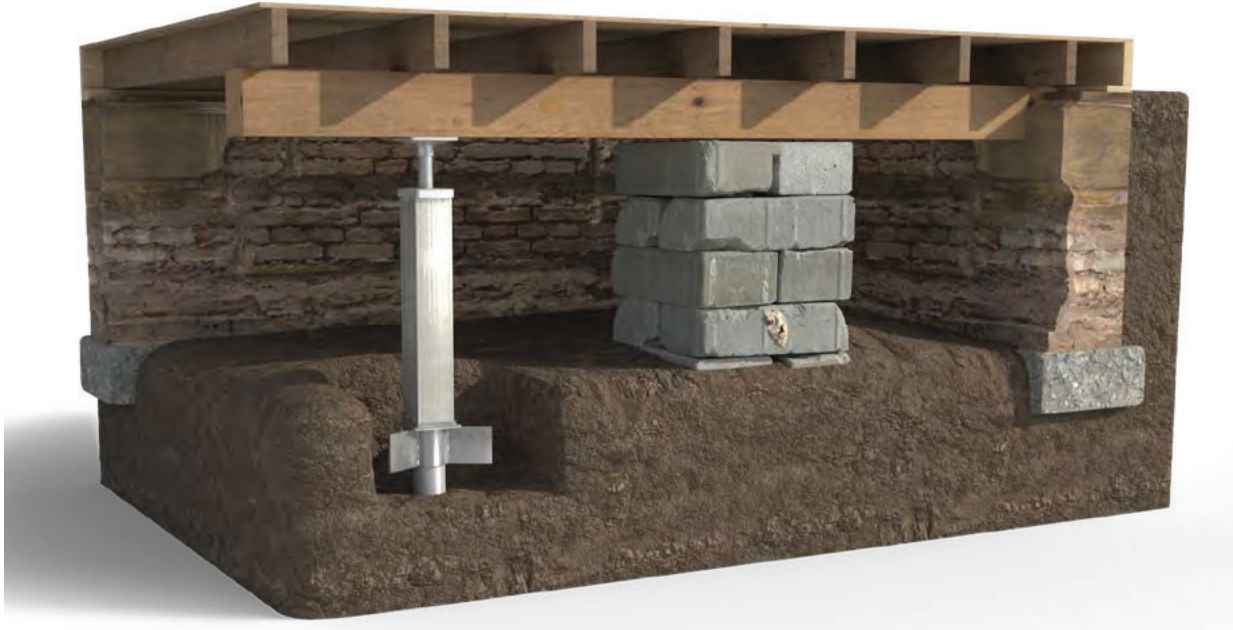
Figure 4.11 Graphic of push pier/SmartJack installation. Backfill around base of SmartJack not shown for clarity. Backfill is required.
